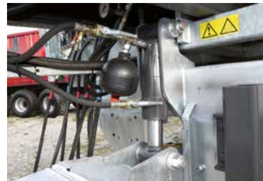
Hydraulic tow bar suspension starting with the ASW256 - trailer height infinitely variable
