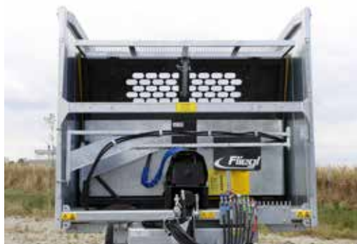
Solid and reliable Push-Off system – no sensitive wearing parts
