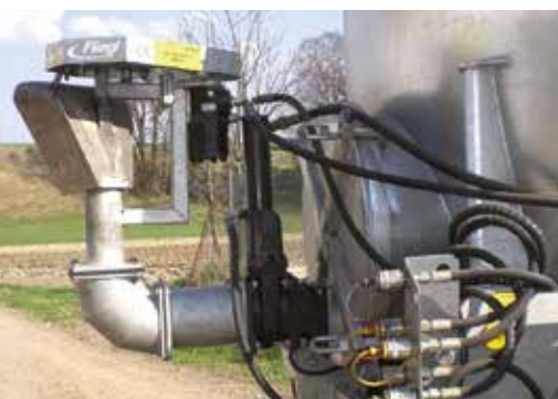
Improved, targeted distribution with the hydraulic auger spreader. Working width 12 to 18 m.
