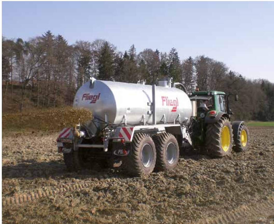
Auger distributor for application of large drops
