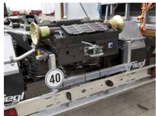
Optional: Extractable underride protection for various container lengths
