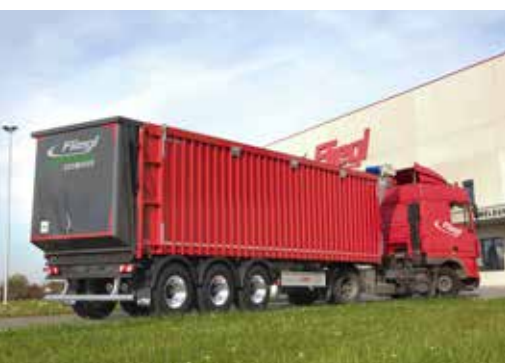
Optimized weight with side panels made from aluminum, Volume 55 m 3 superstructure approx: 7.100 kg
