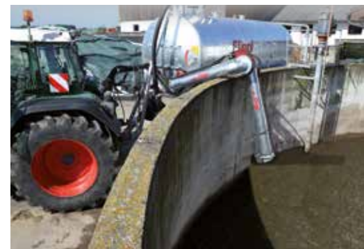
Elefant 8" suction nozzle Left and right possible. Length 5000 mm with quadruple control block Turbo filler and telescopic extension 1500 optional
