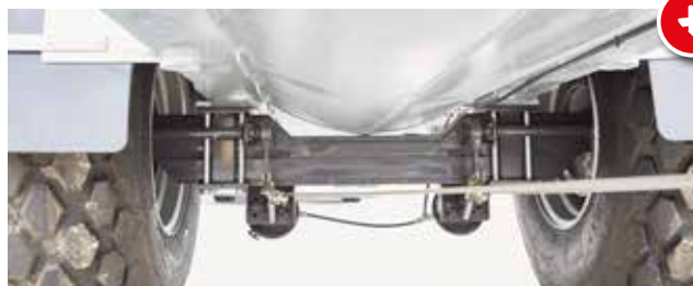
5,000 litres and above with offset axle: Low centre of gravity improves safety on slopes
