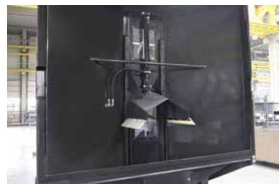
Hydr. manure spreader allows the overloading auger to be completely emptied when loaded
