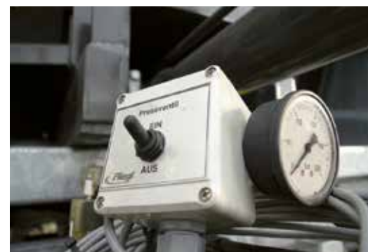
Automatic press valve – the compression of the cargo is automatically pressure controlled
