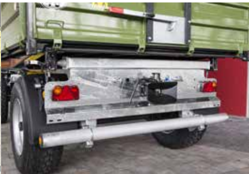
Automatic trailer hitch with hydraulic- and brake connection for a second trailer.
