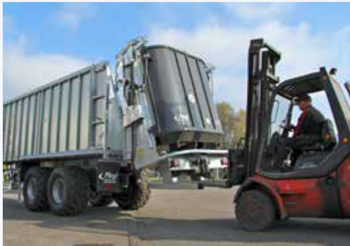
Within 20 minutes the spreader is demounted with a forklift
