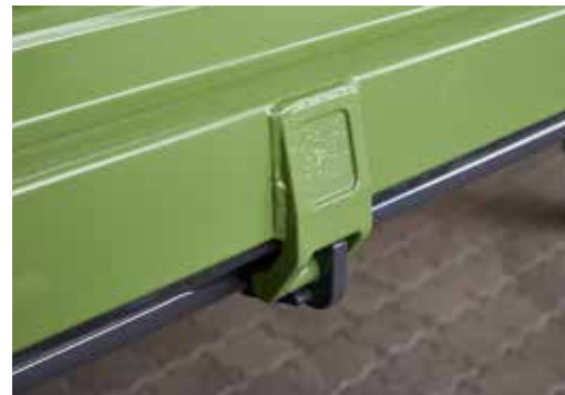
Central side locking - standard equipment available from EDK 60, from 4.500 mm platform length the tippers are locked six times, integral platform profile.
