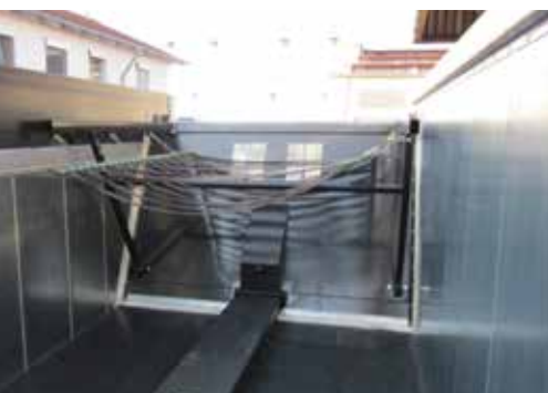
The fall breaker prevents damage caused through dropping the harvested potatoes
