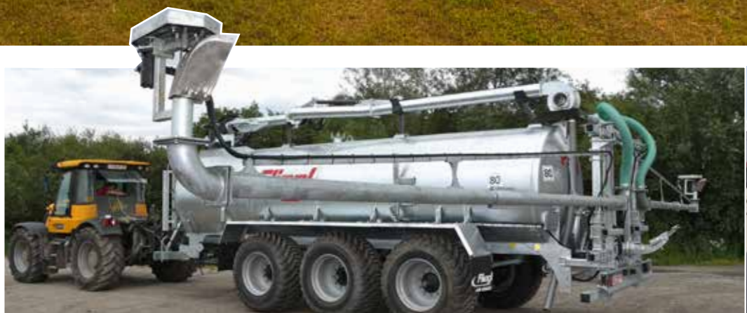
The nozzle bar spreader with a maximum working width of 21 to 30 m
