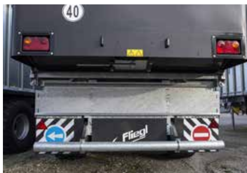
40 km/h-Version with folding underride guard (Germany)
