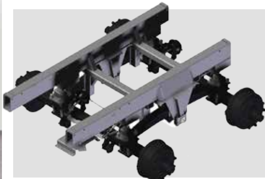
Titan tandem unit for the ground compensation
