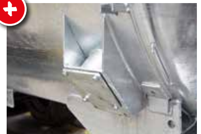
Preparation for connection to turbo filler
