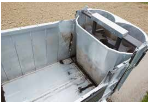
The fully galvanized spreader is in-built as standard. The spreader bearings can be accessed via a central lubrication strip for ease of maintenance.
