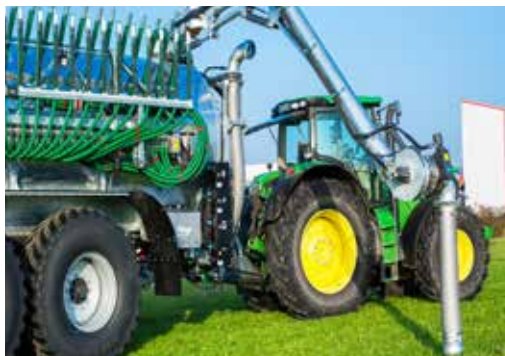
Slurry crane 8" Swivels both sides (180°) Length 8500 mm incl. turbo filler and quadruple control block
