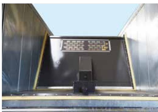
Special sealing of polyetherane: Due to a special sealing at an angle of 45° in the Push-Off mechanism the "Gigant" is absolutely grain tight.
