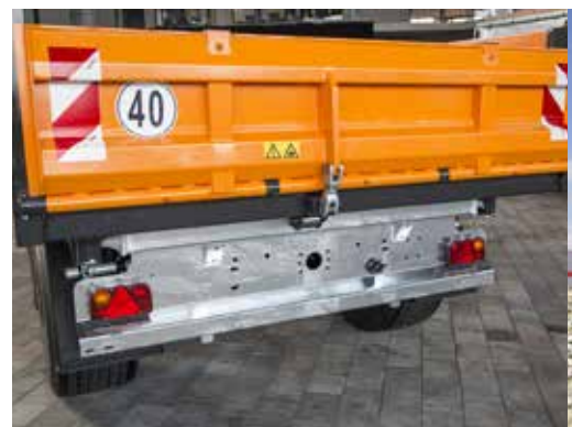
40 km/h version with underrun protection and mudguards
