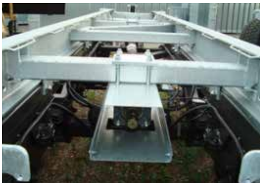
The spreader mechanism is operated mechanically via a driveline
