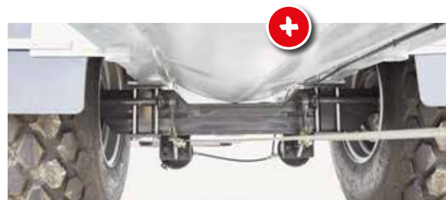
5,000 litres and above with offset axle: Low centre of gravity improves safety on slopes
