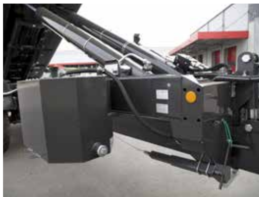
60 l board hydraulic (optional 90 l) driven by PTO driveline with hydraulic pump and oil tank 60-litre hydraulic tank (optional: 90 litres) powered via PTO
