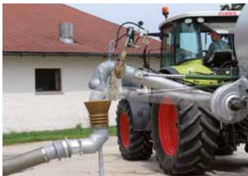
Suction nozzle with 8" turbo filler Left and right possible. With docking station; pressure sequence valve and hydraulic compressor switch
