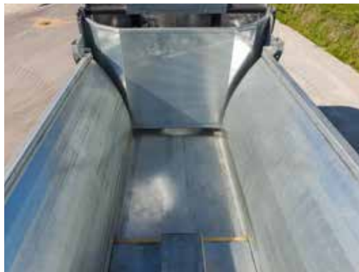
Minimal wear and tear due to hydraulic push system - no scraper floor
