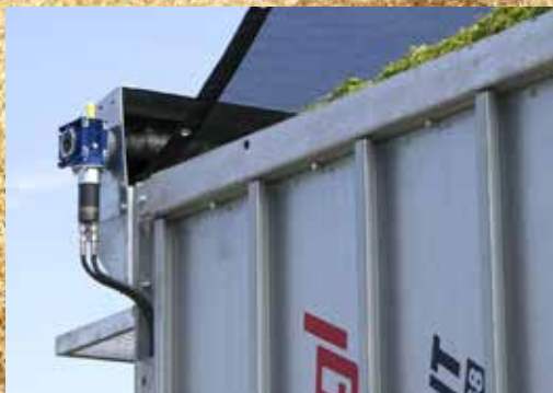
Hydraulically driven oil motor, for the collecting in the covering net
