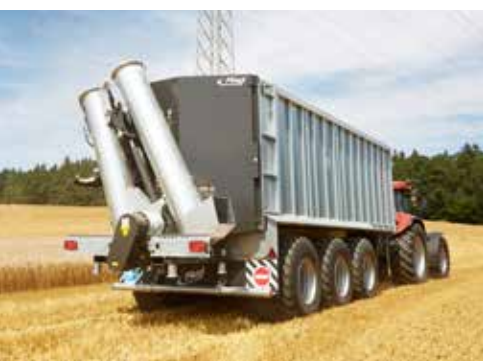
Overloading pipe 400 mm diameter Folds hydraulically
