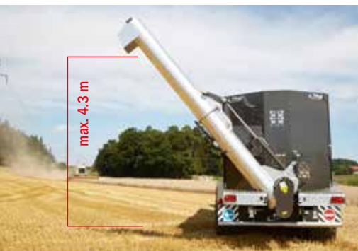
Overloading height 4.30 m (depending on tyres)
