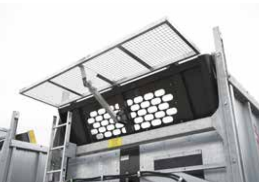
Grin panel extension: Can as standard be adjusted mechanically (hydraulic adjustment is optional).
