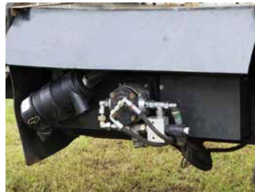
Piston compressor with up to 3 m 3 air capacity
