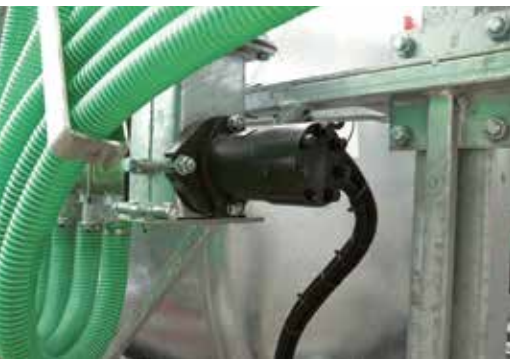
Oil motor for auger dispenser, with interim storage for less wear and a longer service life.
