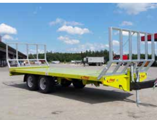
Tandem platform trailer with bale grid and special painting (optional)
