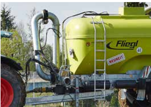
Elefant 8" suction nozzle left or right Length 5000 mm with quadruple control block Optional 1500 mm telescopic extension
