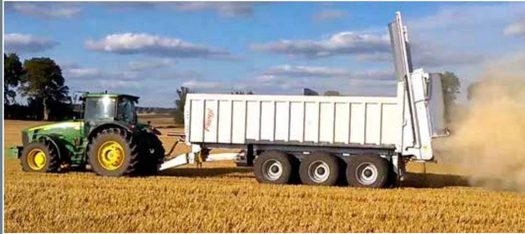
ASW 373 Tiger with protective grille to prevent ingress of foreign bodies
