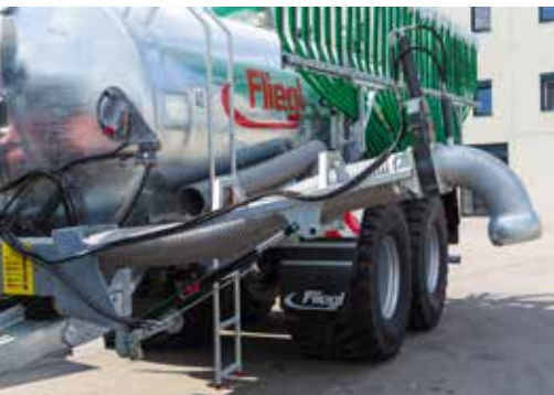
Suction nozzle 8" Left and right possible. With docking station; pressure sequence valve and hydraulic compressor switch
