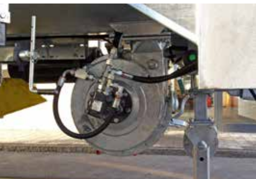
Turbo filler with quick connector (6" or 8") Left and right possible. From 30.5" tyres
