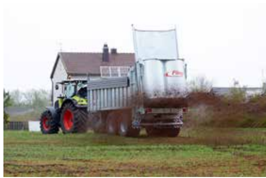
»Profi V2« spreading mechanism with closed rear spreader panel with a spreading width of 18 - 27 m
