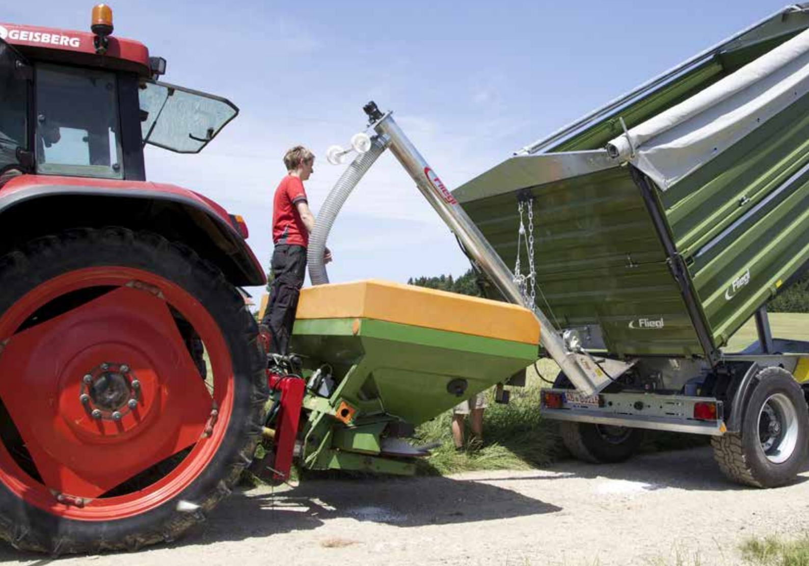
Transfer auger diameter 150 mm, length 3.000 mm and 4000 mm, galvanised or of high-grade steel, easy to assemble, with adjustable cable winches and rotors for transport.
