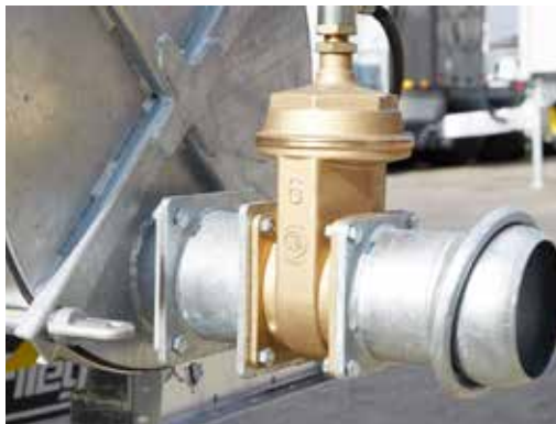
Hydraulic bell valve, robust and resistant to residues (ideal for straw manure)
