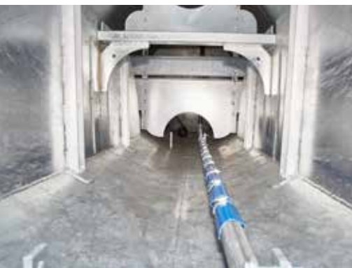
Internal air agitator, only available in combination with compressor. Homogenises liquid manure
