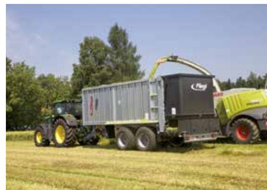
Large rear panel with unloading dispensers. The integrated cross conveyor belt and the beater bars ensure unobstructed feeding in the barn - ejection both left and right
