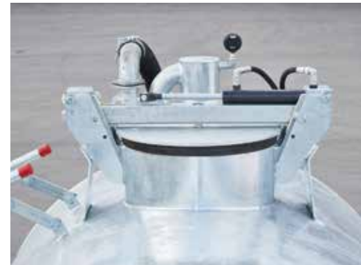
Hydraulic filling dome Available sizes: Ø 500 and Ø 600 mm
