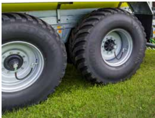
Tyre-pressure monitoring system for field use to reduce soil compression with one and two-pipe system
