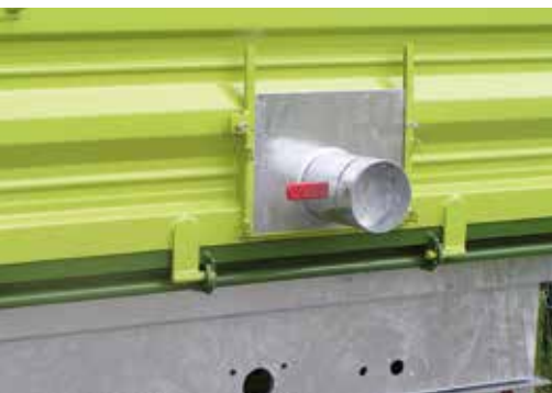
Pipe outlet with outlet support – available from EDK 40.
